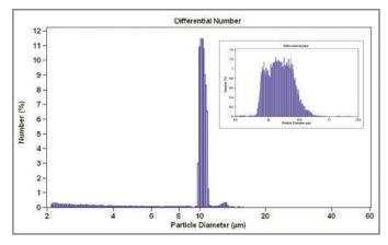
Changes in particle size can be measured in real time thanks to patented digital pulse processing technology. This allows the speed of cell-mediated responses, solutions, aggregates, and dissociation of particles to be analysed.
