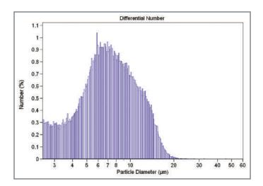
In multiple-aperture mode the software combines data from multiple series of analyses using progressively smaller diameter apertures.
