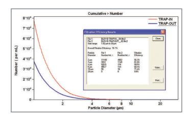
The Multisizer 4e control station memory stores complete information on pulses registered during an experiment. This allows the data to be reanalyzed after an experiment with different particle size range settings to obtain more detailed information on particle size distribution. The instrument not only increases the distribution fragment, but processes and re-analyzes pulses recorded for a given range.
