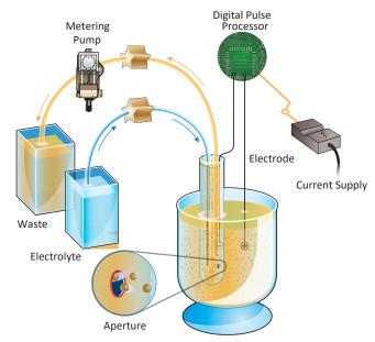
This results in a small change in the voltage in the amplifier, which converts variance in current into a pulse. The height of the pulse is proportional to the particle size and sufficient to give a precise measurement of the particle.
