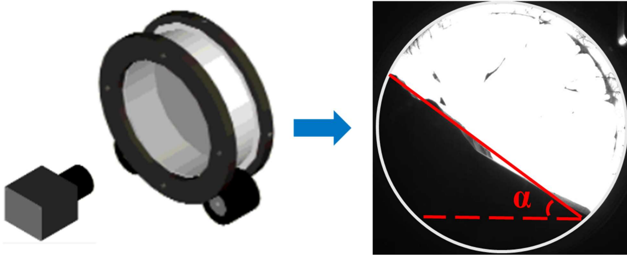
Figure 1. Illustration of working principle of Revolution Powder Analyzer. Avalanche profile of powders is captured by a camera as the drum is rotating. The avalanche angle \alpha is measured by image analysis
