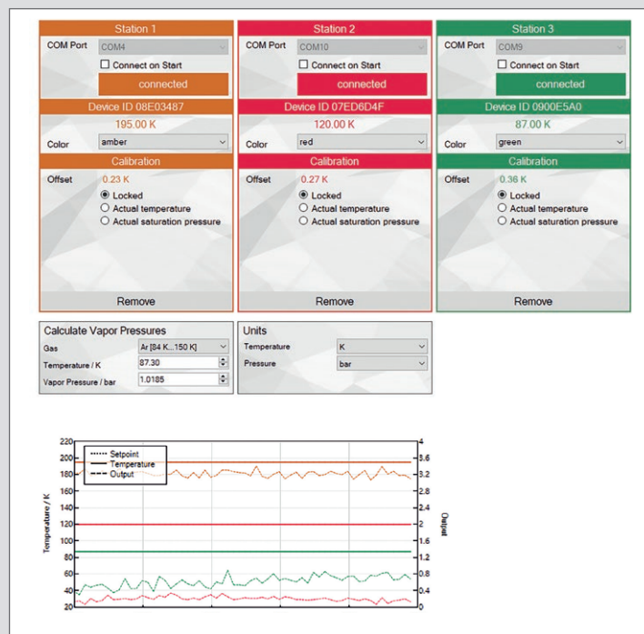
Figure 7 The cryoTune software displays and records the real-time temperature as well as the remaining measuring time with the actual nitrogen filling
