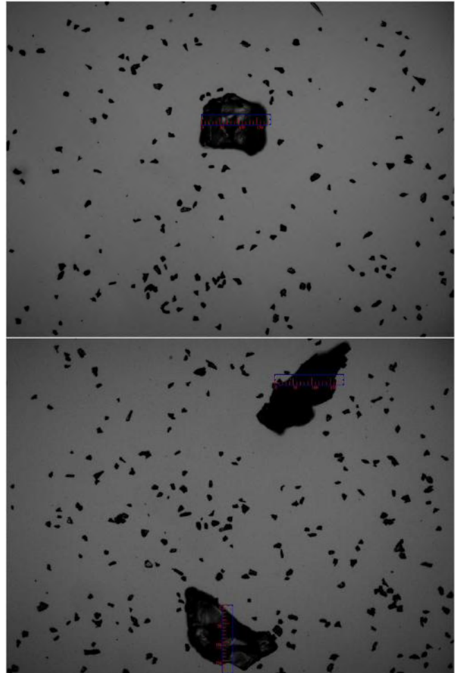
Figure 3. The coarse state of 4#_Mixed via BeVision S1 Image Particle Size Analyzer
