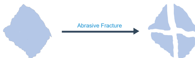
Figure 1. Diagram of self-sharpening behavior of abrasives
