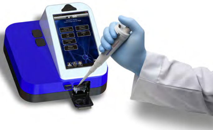
Figure 1 – Orflo's Moxi GO II – Next Generation Flow Cytometer. Image shows user loading a sample into the two-test disposable flow cell. The Moxi GO II is a configurable flow cytometer with a 488nm laser and up to two fluorescence recording channels (2 PMT's with emission filters at 525/45nm filter and 561nm/LP, respectively).
