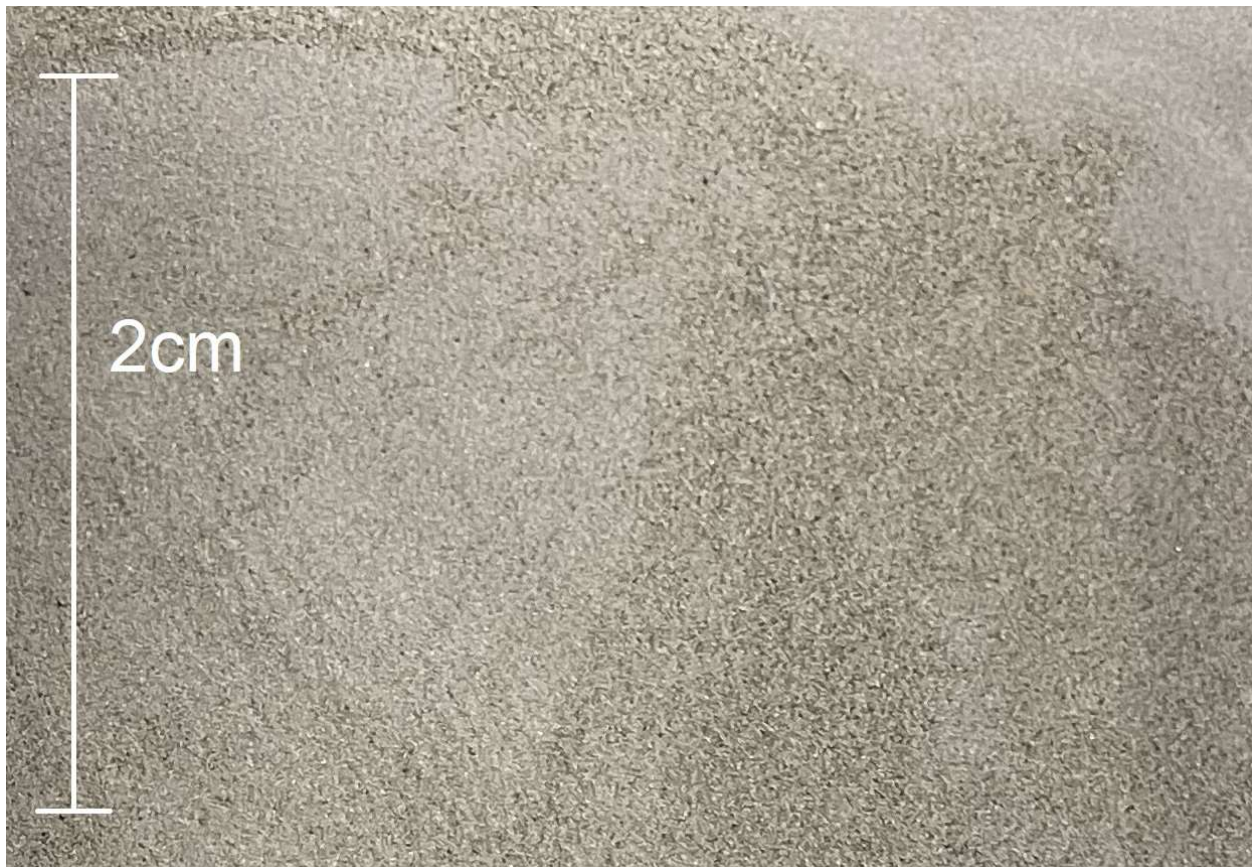
Figure 6. Image of the segregation pan top surface for Set B Recycle after sifting. Larger particles can be seen on the top surface.
