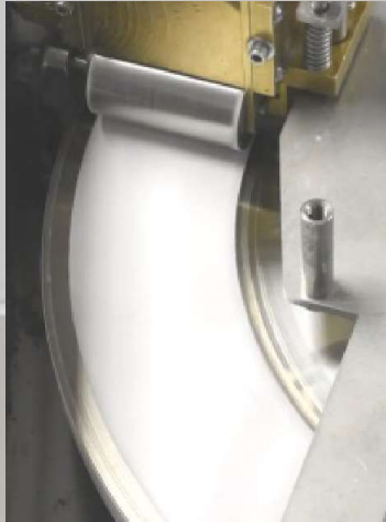
Polymer spread with a counter-rotating roller
