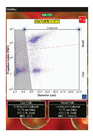
Jurkat cells were analyzed using the new Cell QC App with a PI stain. The Auto-Gating algorithm analyzes results in an accurate, repeatable way to provide the most consistent results possible.
