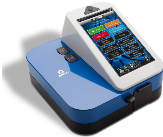
Figure 1 – Orflo's Moxi GO II – Next Generation Flow Cytometer. The Moxi GO II is a configurable flow cytometer with a 488nm laser and up to two fluorescence recording channels (2 PMT's with emission filters at 525/45nm filter and 561nm/LP, respectively).
