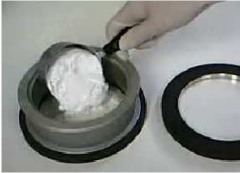
Filling the sample drum
