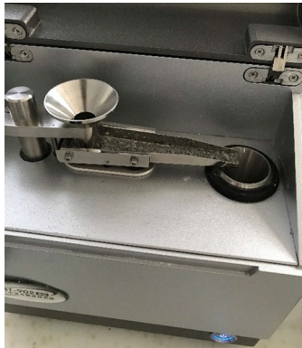
Figure 4. The dry feeder having cement added to the sample tray
